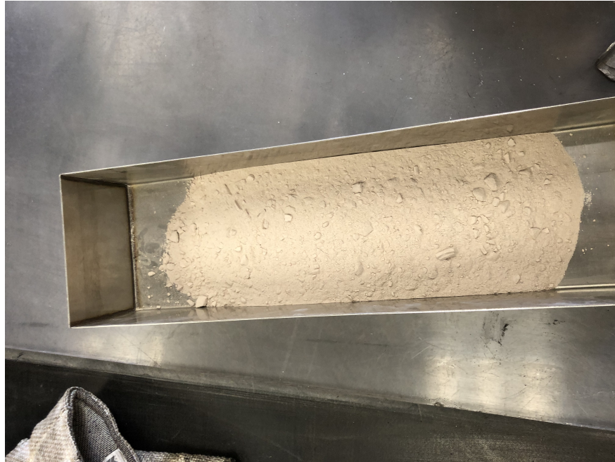
Figure 2: Chalcopyrite ore after splitting
